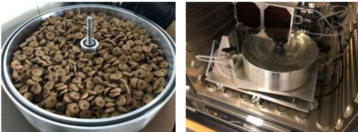
Figure 7. Left: A sample of cat food from VPG in the DTI sample chamber. Right: The same sample chamber mounted in the setup at DTI.
