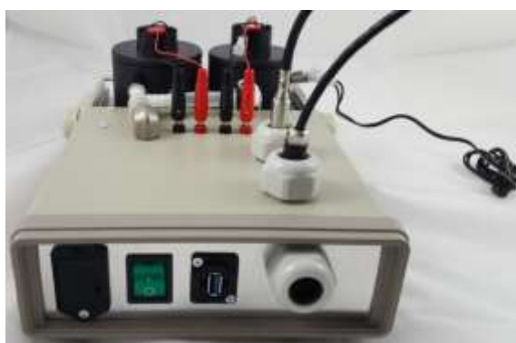
Figure 6 – Field calibrator developed at VTT MIKES
