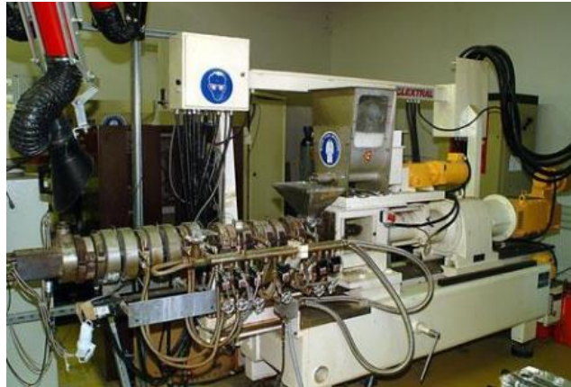
Figure 5: Photo d'une extrudeuse (source extrusion-relative.com)
