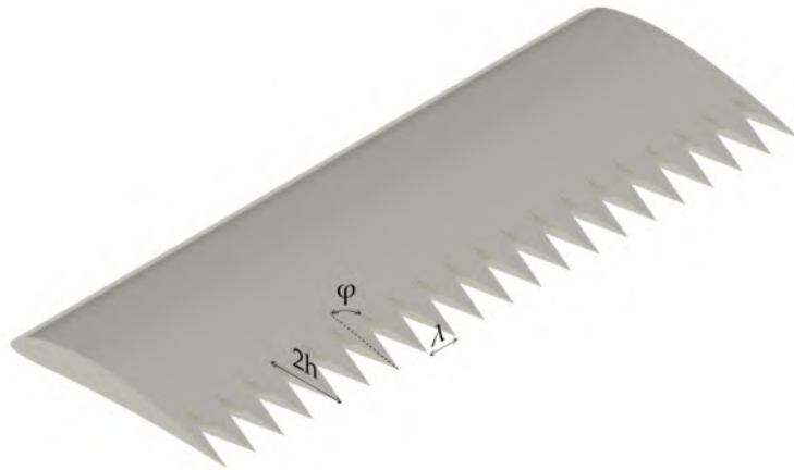
Figure 1.1 – Rendering of a NACA 6412 airfoil with trailing-edge serrations
