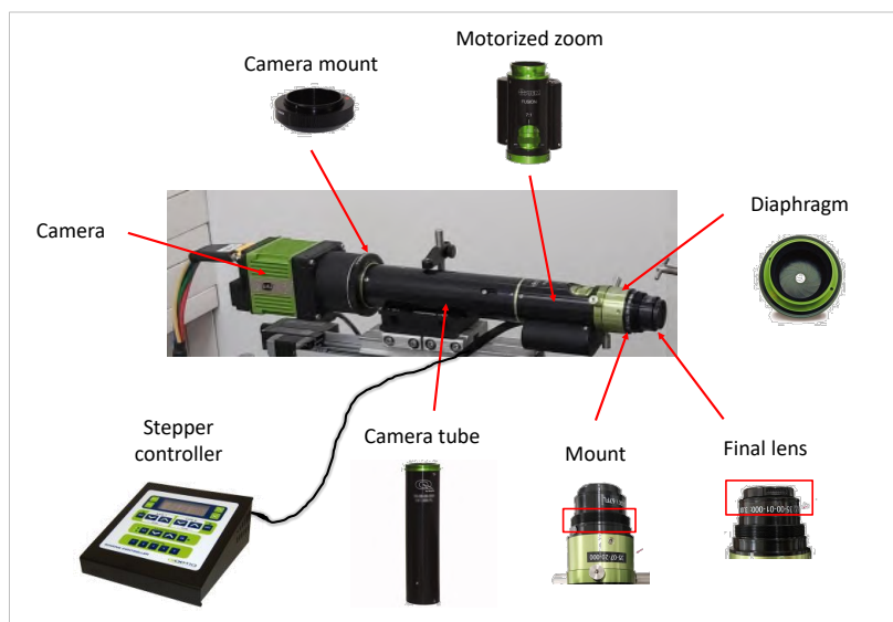
Figure 3.3: Components of the lens system used with the JAI spark camera [111].
