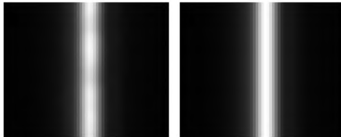
Figure 4.6: Micrometer line before (left) and after (right) vertical averaging of pixel intensities
